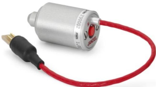
The Cylindrical Probe has spring loads which are user adjustable within one of three ranges. The probe shown here has been factory set to 100 grams per tip, however, the user can increase the load to as high as 150 grams per tip or as low as 60 gram per tip by moving the red Teflon knob towards either the "H" for higher or towards the "L" for lower.
