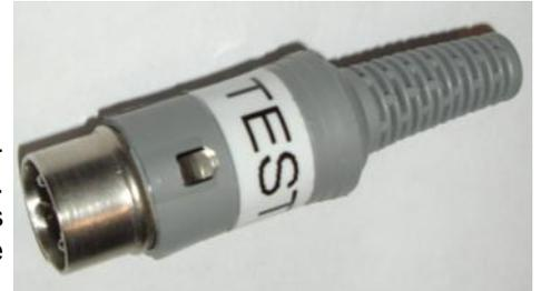
The 100 ohms resistor plug houses a precision resistor which can be used as an external reference to check the functioning and calibration of the HM21 Hand Held Meter. Plugging the 100 ohm test resistor into the HM21 will make the unit respond as if it is measuring a sample. Pressing 'Inc' or 'Dec' will increase or decrease the current. Use these buttons to set the unit to 1mA.
