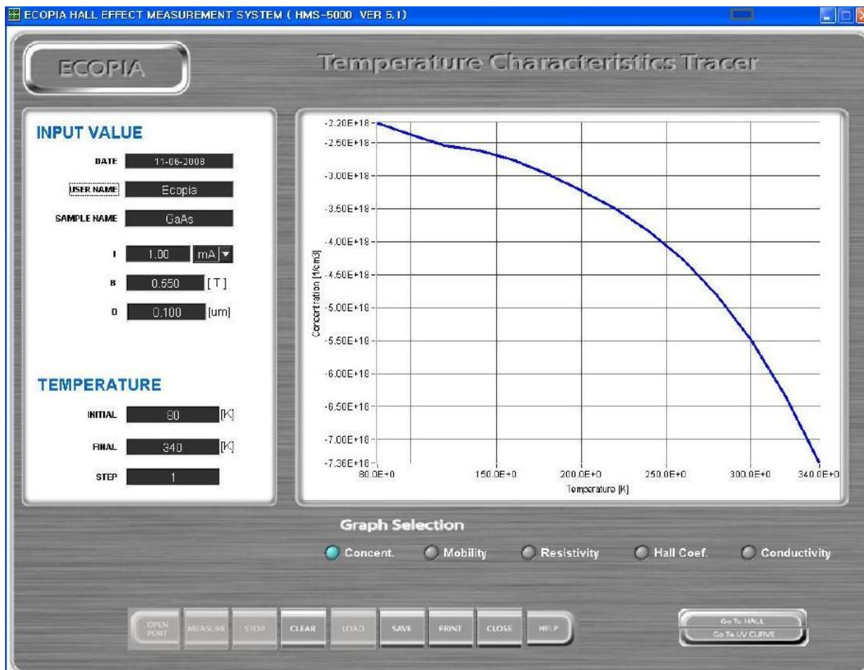
Software displaying Bulk Concentration Versus Temperature in range from 80K to 340K
