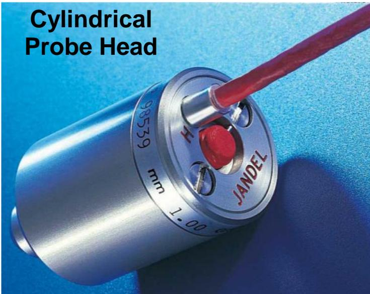
Each Jandel **Hand Applied Probe** includes one **Cylindrical Four Point Probe Head**. The Probe head has a 7" cable which terminates with a Lemo plug. The probe head is available in one of three user adjustable pressure ranges which allows the user to change the tip pressure within the chosen range. Further information about the Cylindrical Probe Head can be seen in the following links:
