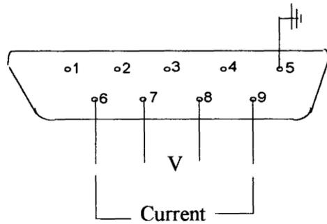
To lead with 180 ° DIN plug on Test Unit
