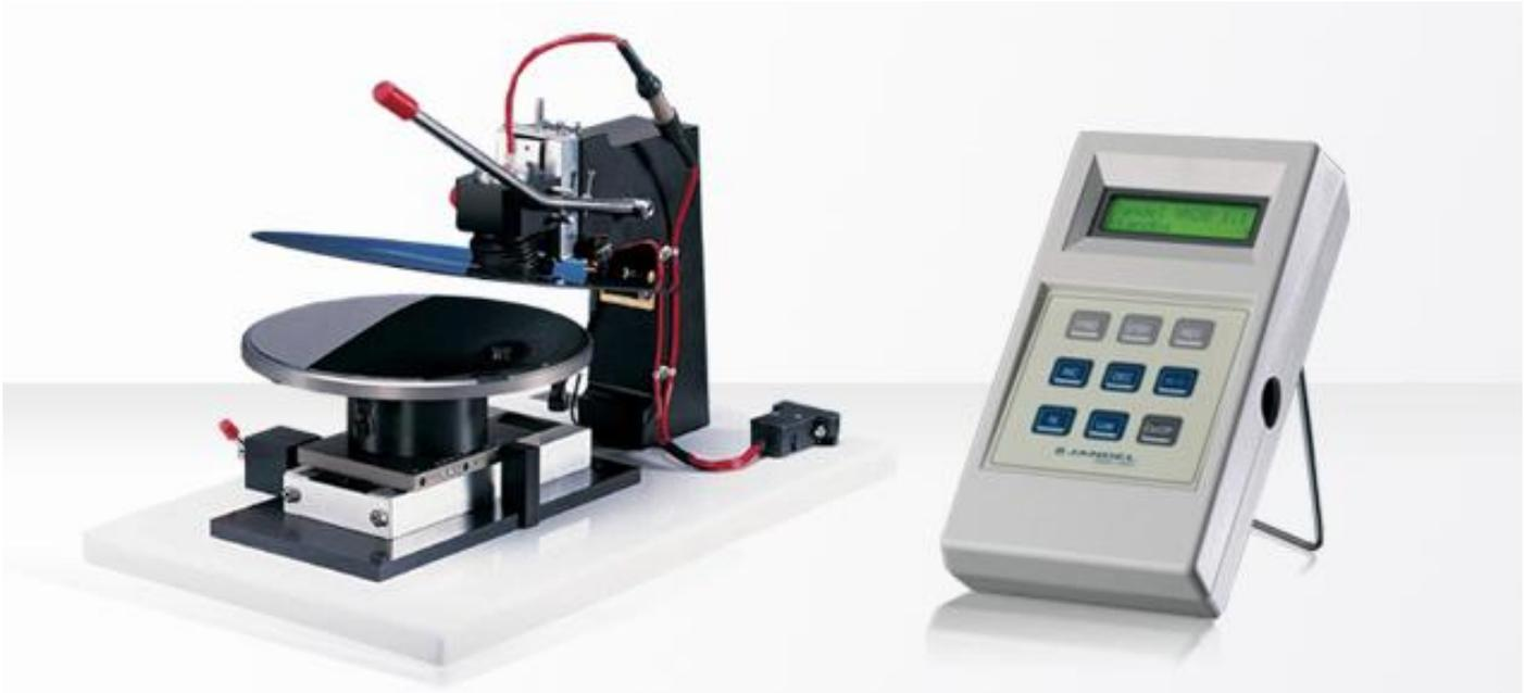
The Multiposition Wafer Probe combined with the HM21 Hand Held Meter Test Unit provides a high quality, easy to use system for measuring the sheet resistance and/or volume resistivity of wafers up to 200mm (8") in diameter.
