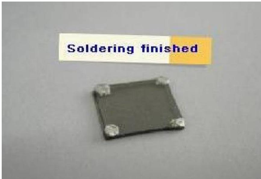
Sample, ready to be mounted onto the spring clip mounting system, or to be wired using the sample board for wire bonding samples.
