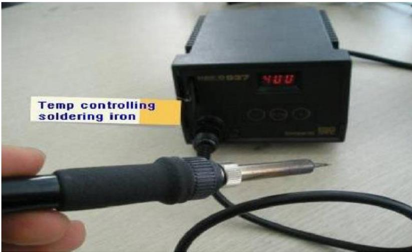
Temp controlling soldering iron
